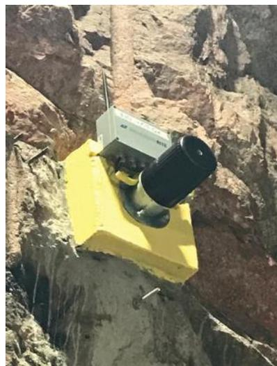
Borehole extensometer with node
