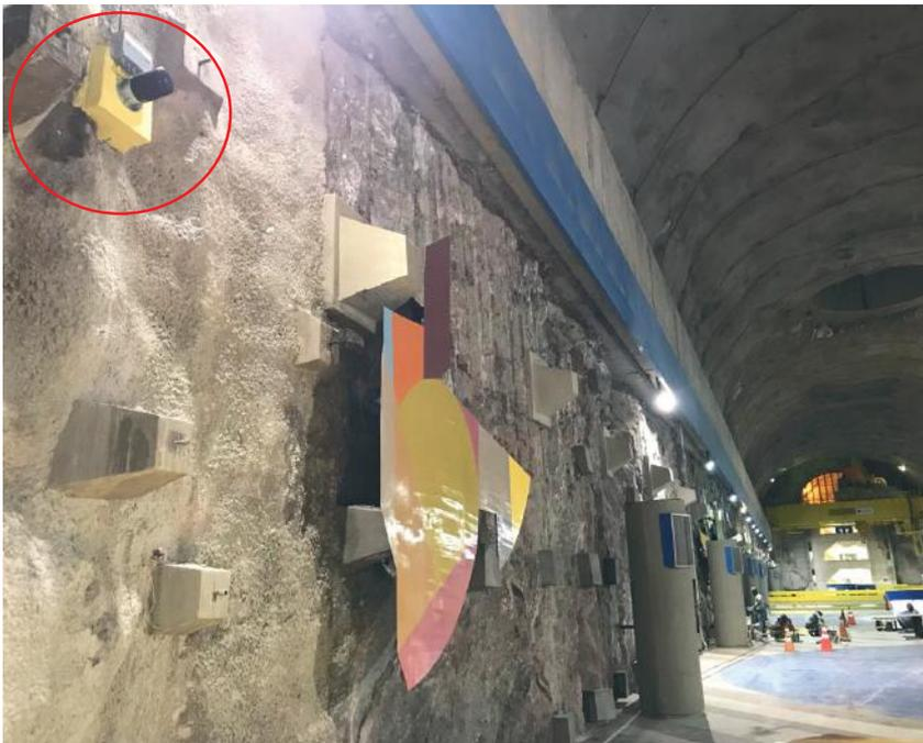
**Borehole extensometer installed with node in underground power house**
